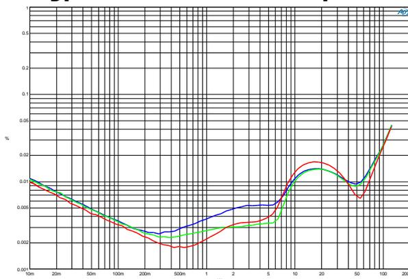
THD+N vs. power at 100Hz (blue), 1kHz (green) and 6kHz (red) (BTL -  $4\Omega$ ).
