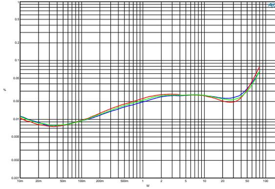
THD+N vs. power at 100Hz (blue), 1kHz (green) and 6kHz (red) (2Ω).
