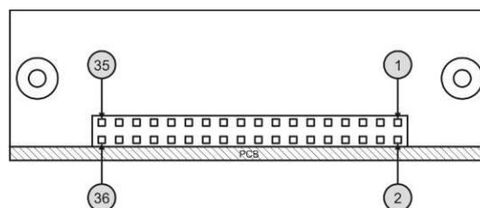
Figure 1. Connector pinning UcD102
