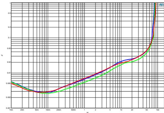
THD+N vs. power at 100Hz (blue), 1kHz (green) and 6kHz (red) (8Ω).
