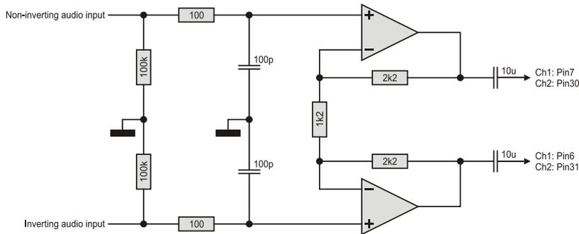
Figure 4. Recommended Input buffer stage.
