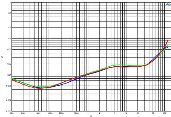
THD+N vs. power at 100Hz (blue), 1kHz (green) and 6kHz (red) (4Ω).
