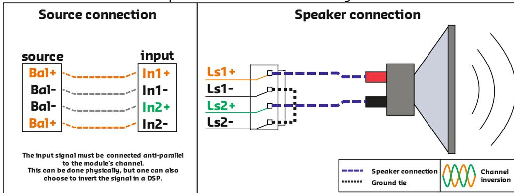
In the graphical representation above, the BTL principle is depicted. By inverting the signal input of the second channel, the output voltage amplitude is doubled. Please note that the negative (GND) output terminals are tied together. On the UcD102 module, this is already implemented in the design and therefore these pins can be left unconnected.
