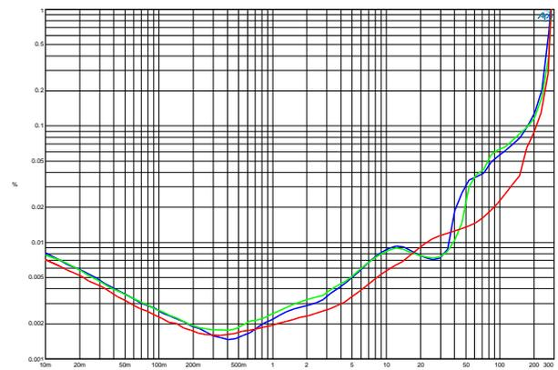
THD+N vs. power at 100Hz (blue), 1kHz (green) and 6kHz (red) (BTL -  $8\Omega$ ).
