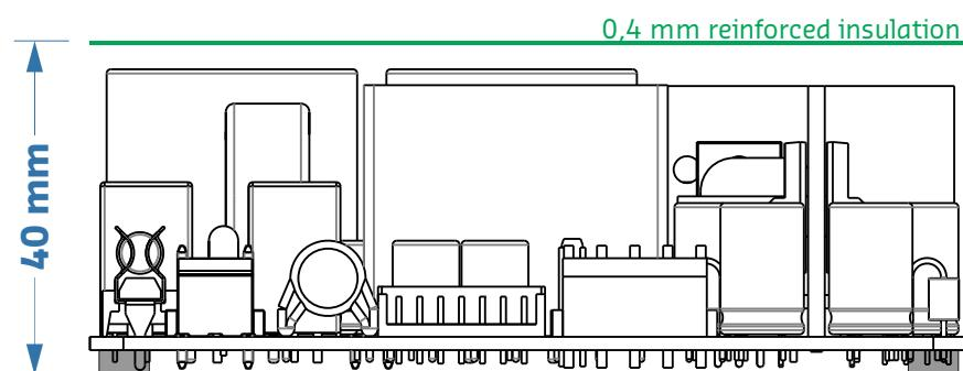
Note: In all cases, provide a minimum clearance of 3 mm over the primary capacitors, to avoid blocking the correct opening of the pressure relief vent.
