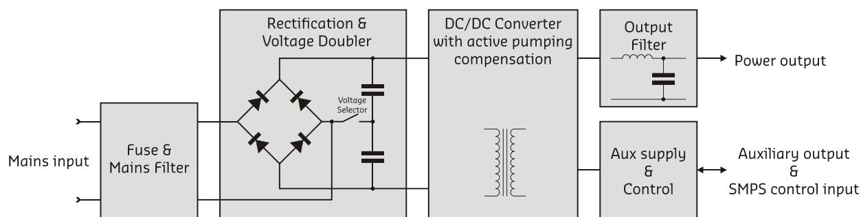
Conventional Switch Mode Power Supplies are commonly unsuitable for audio purposes due to poor peak power capabilities and the inability to handle reversed currents generated by Class D amplifiers as a load. The Hypex SMPS400 achieves these things by using an advanced over current protection circuit, a highly efficient 2 quadrant DC/DC converter which is capable of handling reversed currents and has a peak power handling of many times its rated power.
