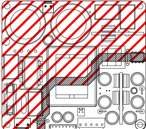
This is a Safety Class 2 device. When mounting the module in an enclosure, a minimum safety distance of 6mm from the SMPS to all possible conducting parts must be ensured to keep compliance with Safety Class 2. All parts enclosed by the red line carry hazardous voltages. This includes parts on the top and the bottom of the board. Only use insulated spacers and fasteners in the red area.
