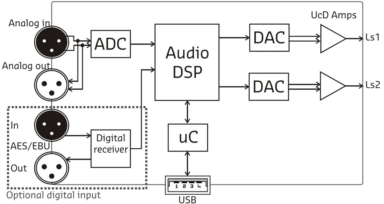
Figure 3: Block diagram
