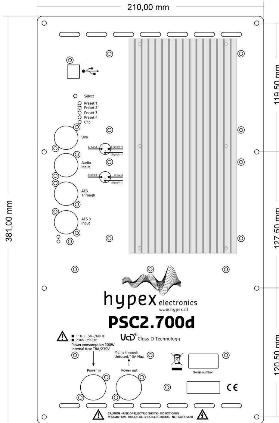
Figure 13: Plate amp 2xUcD700Watt
